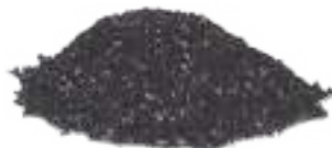
GAC 12x40, 6x12, 8x16 Iodine adsorption 1200
